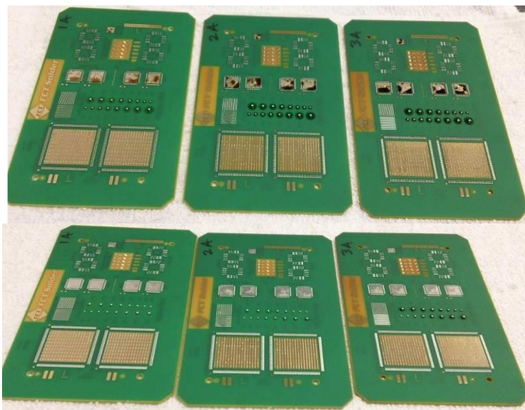
Figure 9 - Reflowed solder paste before (top) and after (bottom) soaking in water for 5 min. The number of reflow cycles increases from left to right (1, 2, and 3)
